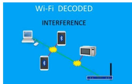
Interference: The 2.4 GHz band has become very noisy in urban areas due to the high penetration of WLAN. Also, there is a lot of interference from other devices that are communicating in the same frequency range, such as microwave ovens, cordless phones, and Bluetooth devices. The 5 GHz band, on the other hand, gives the advantage of low interference.
